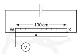
The potential difference (p.d.) between W and X is 1.5 V.
