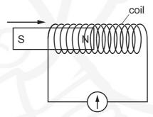
The needle of the galvanometer moves.
