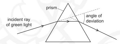
When a ray of white light is incident on the prism, it separates into the colours of the visible spectrum.
