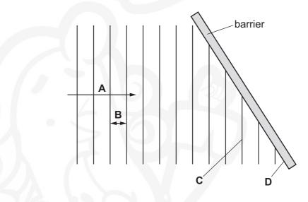
**22** A vibrating object produces ripples on the surface of a liquid. The object completes 20 vibrations every second. The spacing of the ripples, from one crest to the next, is 3.0 cm.
