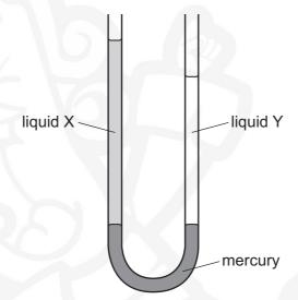
Which row compares the pressure exerted by liquid X and by liquid Y on the mercury, and the density of liquid X and the density of liquid Y?
