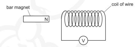
The N-pole of the magnet is moved quickly towards the coil. The voltmeter shows a reading of +10 mV.
